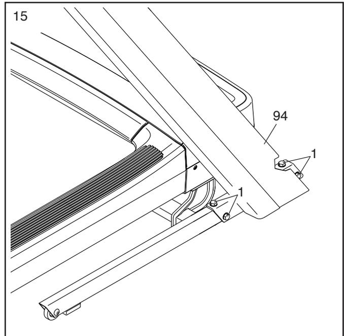
16. Identify the Right Base Cover (98). Slide the Right Base Cover under the Upright Wire (92) and onto the Base (101). **Make sure that the Right Base Cover is under the Upright Wire.**
