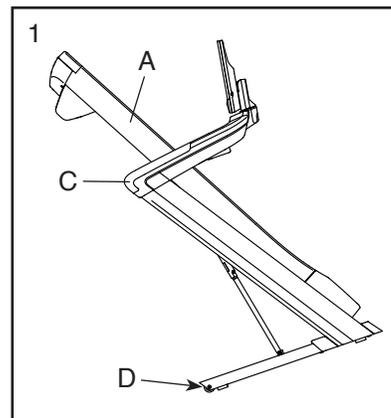
2. Pull back on the handrail (C) until the treadmill will roll on the wheels (D), and carefully move it to the desired location. **CAUTION: Do not move the treadmill without tipping it back, do not pull on the frame, and do not move the treadmill over an uneven surface.**
