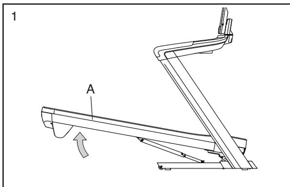
2. Raise the frame (A) until the storage latch (B) locks in the storage position. **CAUTION: Make sure that the storage latch locks.**
