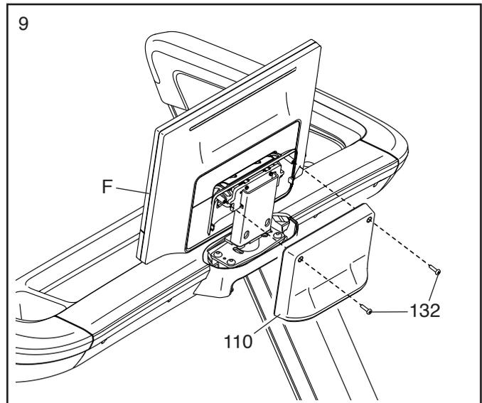
10. Tilt the top of the console assembly (F) in the direction shown by the arrow as far as you can. Then, attach the Lower Pivot Cover (34) to the console assembly with two #8 x 5/8" Screws (132).
